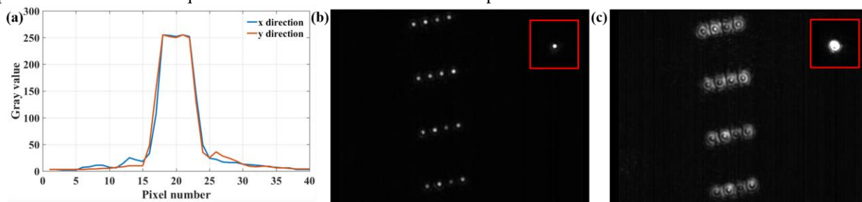
Fig.3 (a) Intensity profile of a single spot. (b) Measured far-field pattern of the grating emitter array. (c) Measured far-field pattern of grating emitter array by de-focusing the device lens. Insets of (b) and (c): Beam pattern with only one emitter switched on.
